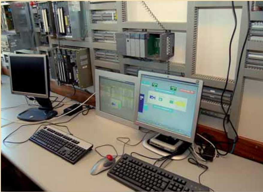
Figure 2: InTouch HMI clients.
