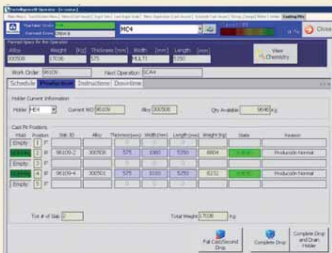
Figure 1: Production tab where the operator can see the work order's production planning and respective attributes.
