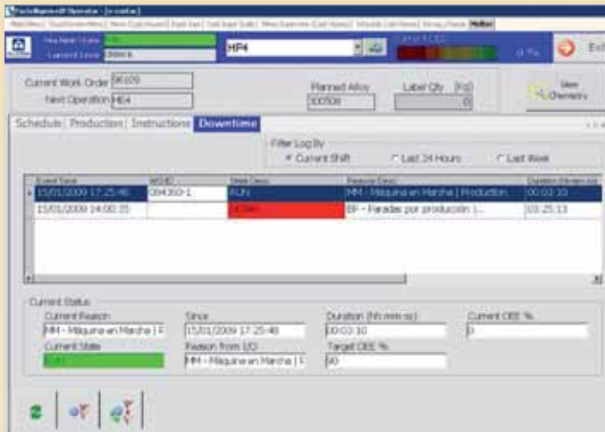
Figure 2: Downtime tab showing the list of latest working status of the machine and its duration, depending on the filter chosen.
