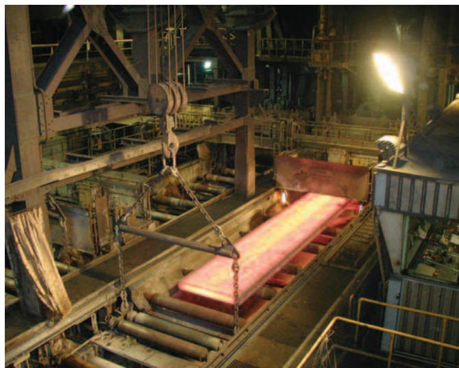
Alloyed steel is cast into slaps continuously
