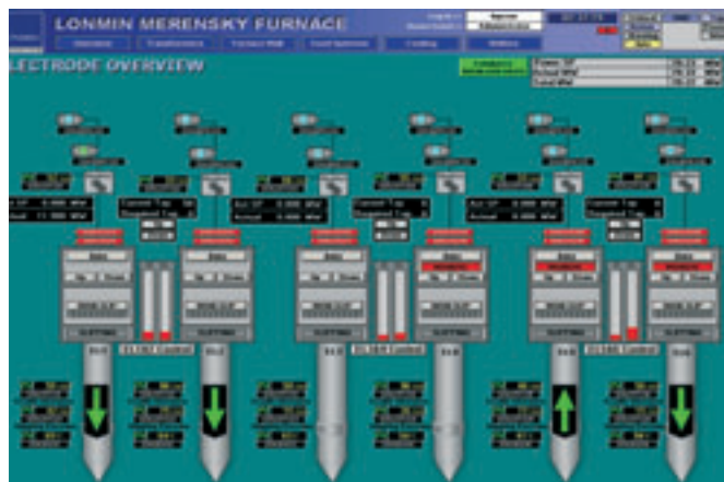
Figure 3: InTouch HMI screen showing the Merensky furnace, which consists of six in-line electrodes operating at a maximum of 9MW. The average operating temperature of the matte is 1280 °C and the slag 1450 °C.
