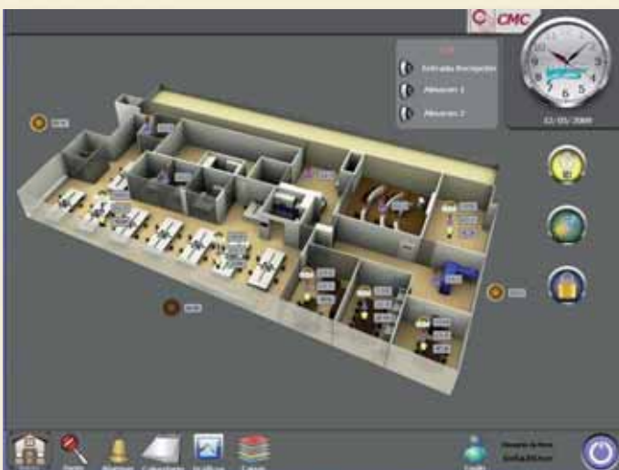
Figure 1: Office synopsis showing the temperature level controlled by Wonderware System Platform.
