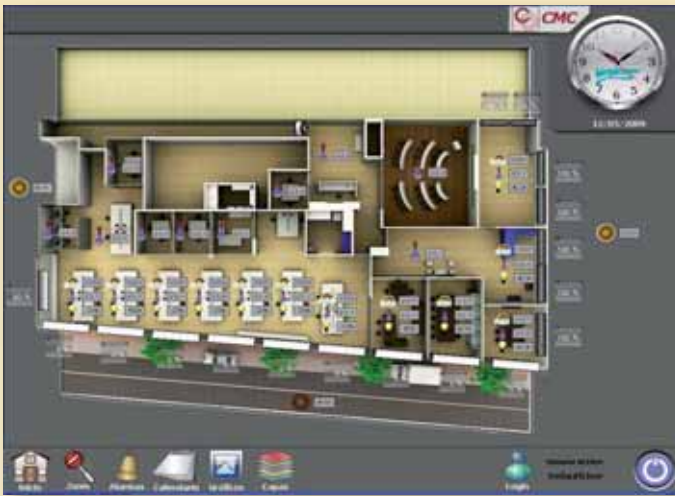
Figure 2: General view with all lighting system, air conditioning and shutters.
